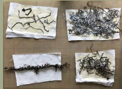
Figures 41-42. Material experiments with seagrass ( Zostera marina ): coiling, spinning and winding, mixing with latex.
